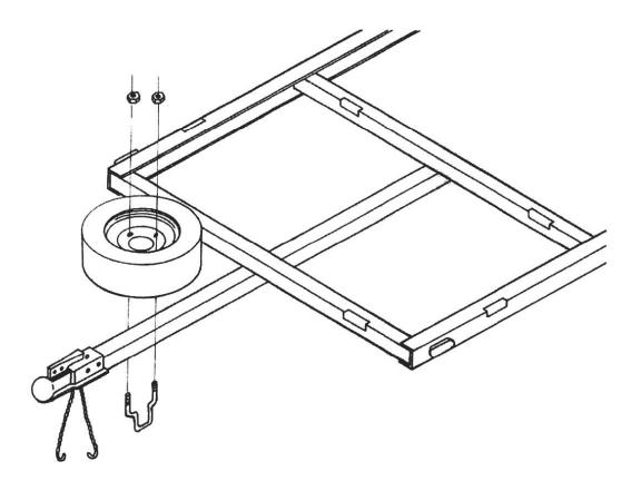
Place "U" holder under towbar and go through two holes on wheel rim, lock nuts with same depth, do not make the tire swing.
